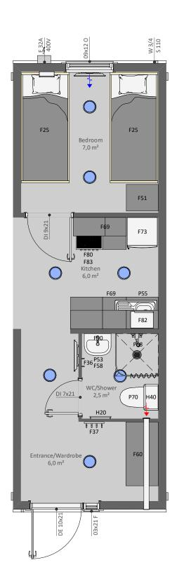
**EV21R** is a functional EVAC module with one living/bedroom, kitchen with dining area, WC with a shower and an entrance/wardrobe room. Can be connected to other our EVAC and site hut modules, especially with the module EV22R
