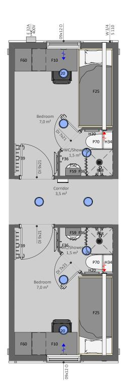
**EV01R** is a functional EVAC module with two bedrooms, two WC with a shower and a corridor in the middle of the module. Can be connected to other our site hut modules
