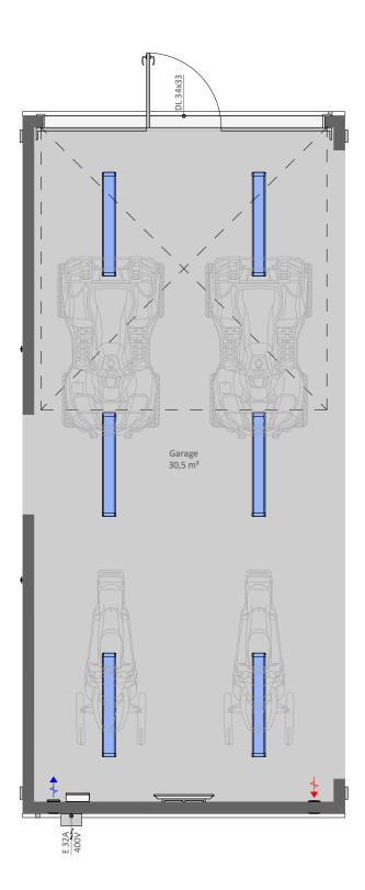
GA10WL is a single open space wide garage module without a wall on one long side, can be connected to other our site hut and garage modules
