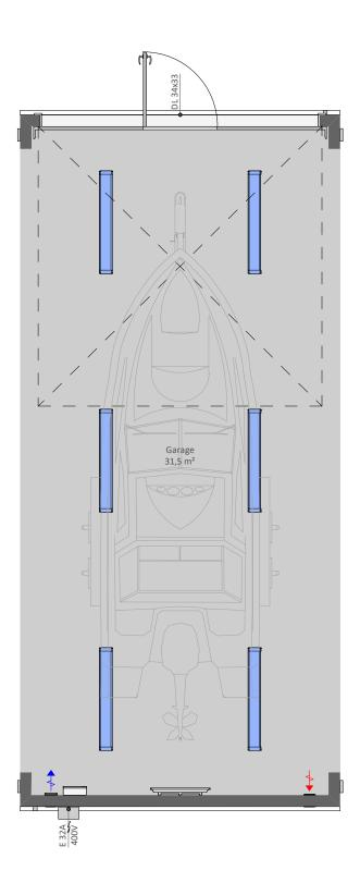
**GA00W** is a single open space wide garage module without walls on the long sides, can be connected to other our site hut and garage modules
