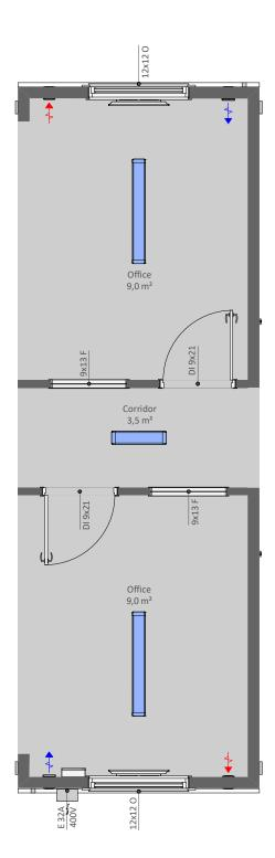
K12HG2D2 is a open space office module with two office rooms and corridor, without a wall on one long side
